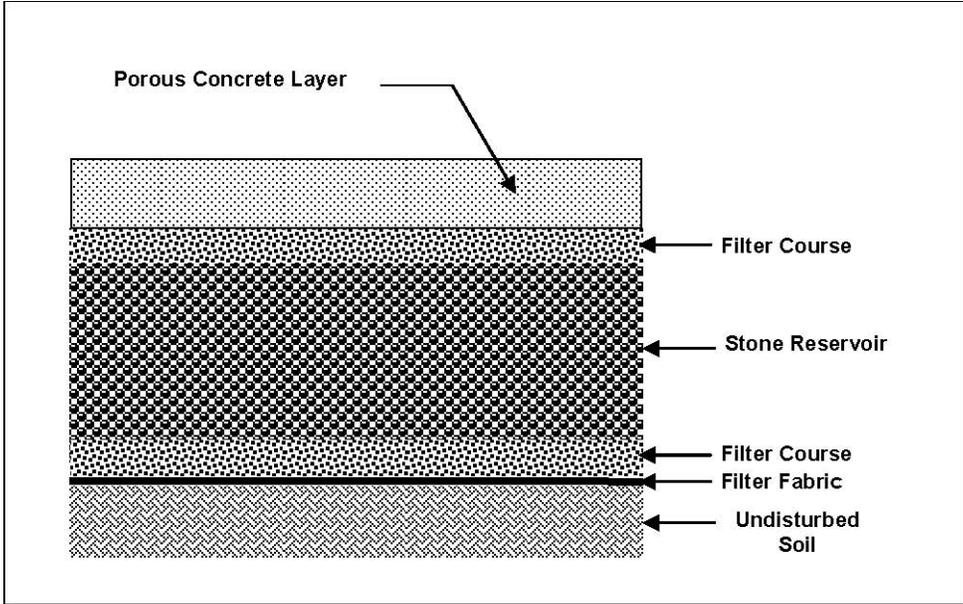
**Figure 2.2.24-1 Porous Concrete System Section**
