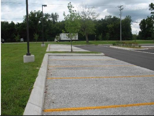
**Description:** Porous concrete is the term for a mixture of coarse aggregate, portland cement and water that allows for rapid infiltration of water and overlays a stone aggregate reservoir. This reservoir provides temporary storage as runoff infiltrates into underlying permeable soils and/or out through an underdrain system.
